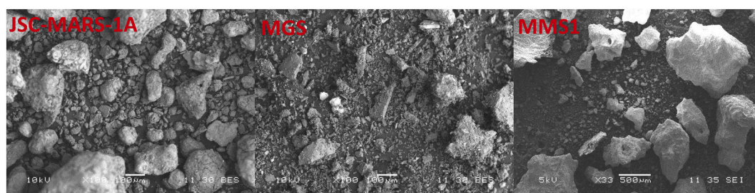
Fig. 1. Scanning Electron Microscopy (SEM) images of the MRS utilized in this study. Left to Right: JSC-Mars-1A, MGS-1 and MMS-1. These images were collected from mixed particle size samples.
